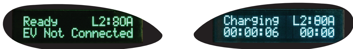
Figure 1. Examples of the QuadZilla LCD Codes
